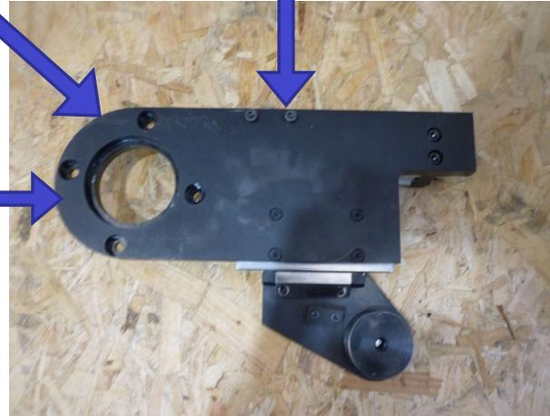
Loosen these screws to remove the tube assembly from its support.
